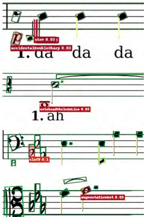
Figure 6: Four cropped visualisation samples of predictions made by an ensemble. The colour of the bounding box indicates the model’s confidence (green means high confidence, and red means low confidence). For symbols with a confidence score below 30%, we plot not only the coloured bounding box but also the assigned label as well as the confidence score.
