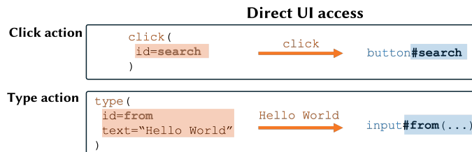
Fig. 6. Common direct UI access actions, referencing the HTML element by its id attribute.
